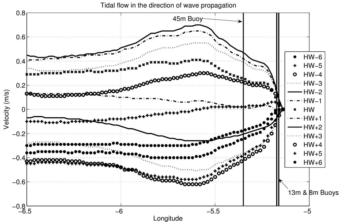
Figure 8. Spatial and temporal variations in tidal flow in the direction of wave propagation at latitude of  $50^{\circ}21'N$  (Perranporth). Note that the locations of the Perranporth wave buoys are shown by the vertical lines and the coast is located on the right hand side of the diagram where the current velocity vectors converge to zero.
