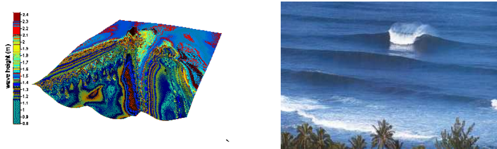
Figure 2: Wave decay along the lane. Left: Wave height special distribution where one can see a strong amplification at the sea board of the reef followed by an also strong decay along the lanes. Right: An example of this situation in nature.
