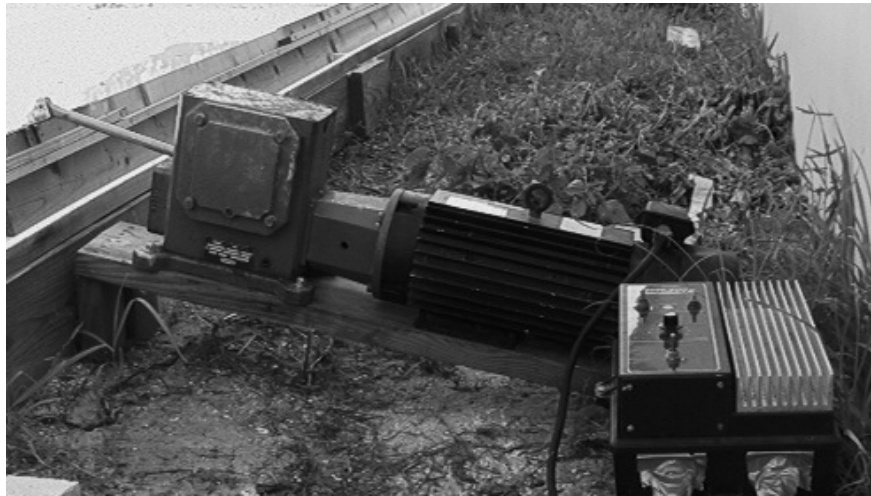
Figure 4 – Wave generator paddle, motor, and controller.
